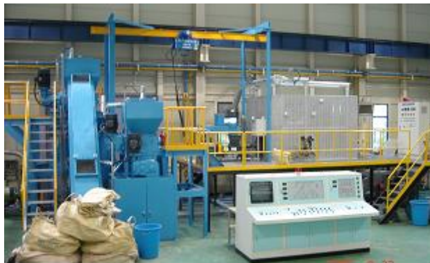
Waste FRP vessel melting system
