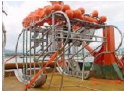
Tow-type survey system and net-fishing gears (1,000m depth class)
